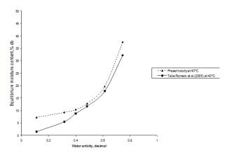
Figure 2. Comparison of sorption isotherms of solar-dried mango slices at 40°C with published data
