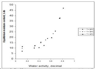
Figure 1. Equilibrium moisture content versus water activity at the different drying temperatures (20, 30 and 40 °C)
